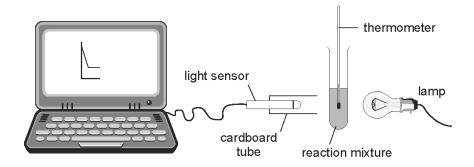
5cm³ of dilute hydrochloric acid was added to 10cm³ sodium thiosulfate solution at 60°C and the light intensity was measured over time. The results are shown on the grid below.
